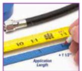
Measure the sleeving and mark the measurement with a pen or marker. Add an additional 1 1/2 - 2 inches and cut the extended length of sleevina. Push the sleeving down over itself and the tape and keep pushing until the other end of the sleeving falls into place at the far end of the application. If there are any sharp edges or loose wires on the ends, temporarily wrap them with tape to avoid snags.
