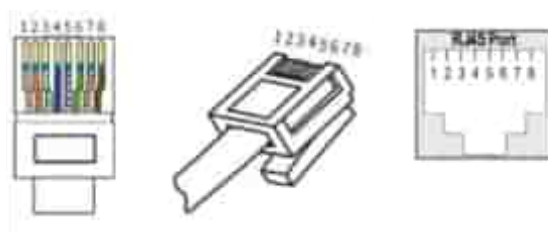
Figure 2-12 "Inverter CAN/RS485" port pins
